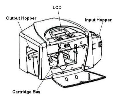
**Reviewing the Printer (front view; Cartridge being installed)**
